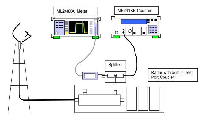
Figure 1. Typical Pulse Radar Measurement Set Up
